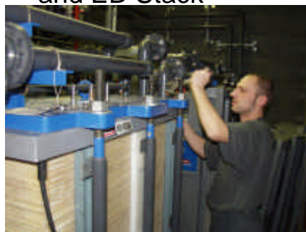
Pump unit of the 20 m 2 plant with sample valve battery at the right side and ED Stack
