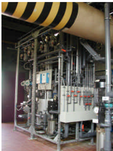
Pump unit of the 20 m 2 plant with sample valve battery at the right side and ED Stack
